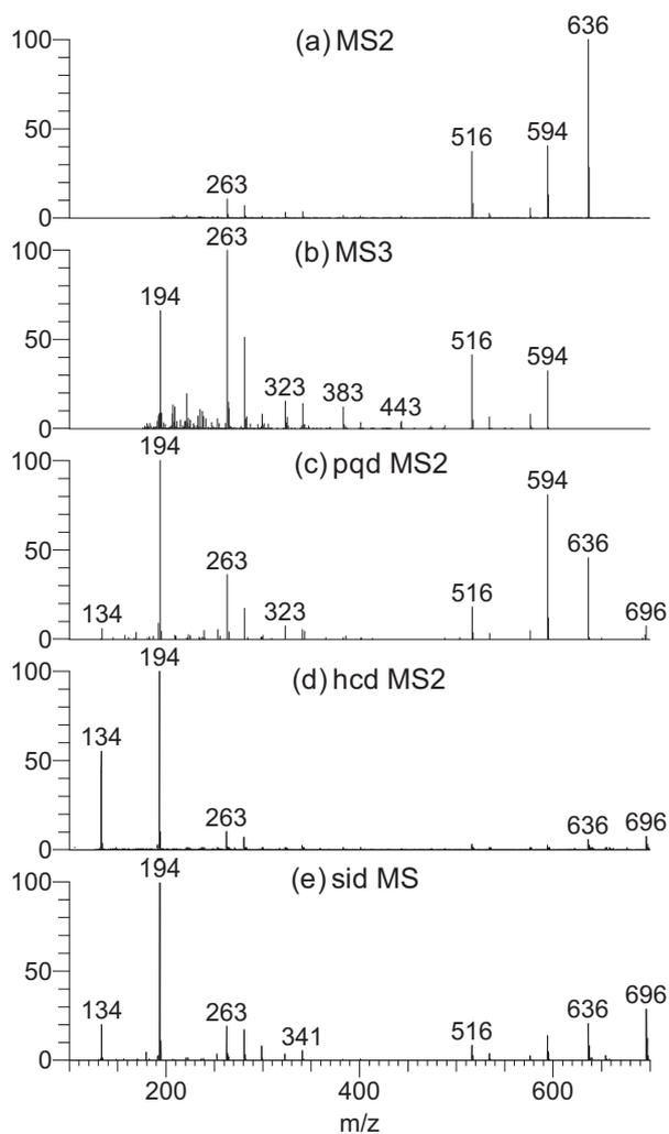
**Fig. 3.** Collision induced dissociation spectra of protonated 2'-deacetoxyaustrospicatine (at  $m/z$  696). (a) MS<sup>2</sup>, (b) MS<sup>3</sup> ( $m/z$  696 → 636), (c) pqdMS<sup>2</sup>, (d) hcdMS<sup>2</sup> and (e) sidMS showing generation of the APPA ion at  $m/z$  194.
